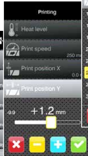
Printing offset y slide control for fast adjustment +/- keys for fine adjustment
